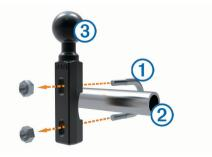
2 Tighten the nuts to secure the base.
