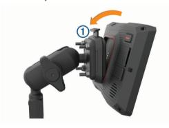
**2** Push the top of the device forward until it snaps into place. The latch ① on the mount stays up after you insert the device.
