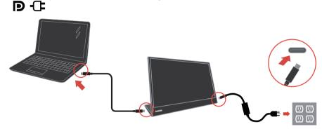
2) Connect Type-C power adapter to the left or right side of M15 and connect M15 to the mobile phone with a USB-C cable.
