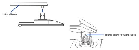
③ Install the Stand-Base to the Stand-Neck and then tighten the 'thumb screw' to secure them.
