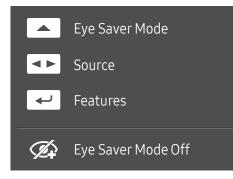
The Direct Key Guide screen shows if Eye Saver Mode is enabled. ( : On, : On, : Off)
