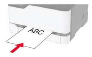
• Load letterhead with the printable side facedown and the top edge entering the printer last for two-sided printing.
