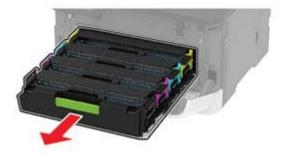
**5** To avoid stray toner contamination, place a sheet of paper on top of the print cartridge tray, and then insert the print cartridge tray.
