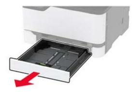
**2** Remove the used manual feeder.
