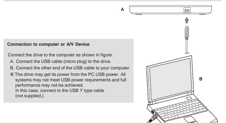
**NOTICE** In case of computers/laptops, a single USB port might not supply enough power to operate the product. If this happens, connect both USB-A plugs (**1** and **2**) of the USB-A power/data cable (H).
