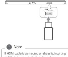
If HDMI cable is connected on the unit, inserting a USB device may be limited depending on a USB device shape.
