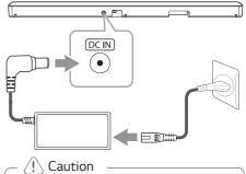
Only use the AC adapter supplied with this device. Do not use a power supply from another device or manufacturer. Using any other power cable or power supply may cause damage to the device and void your warranty.
