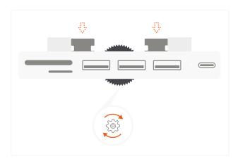
3 Turn the knob in opposite direction. Check that the Clamp Hub is securely fastened to your iMac.
