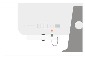
6 USB-C port can be used for data transfer only. Charging through USB-C port is not supported.
