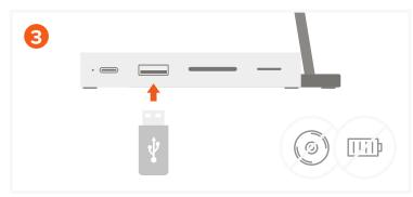
Use the USB-A data port to connect USB devices up to 10 Gbps. Does not support charging or CD readers, including Apple USB SuperDrive.
