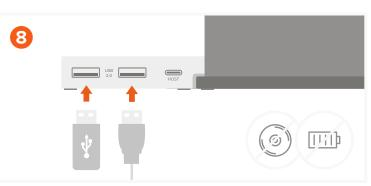
Use 2 USB 2.0 data ports (480Mbps) on the back of the hub to connect USB devices.
