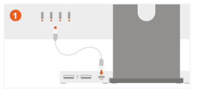
Connect the Hub to one of your iMac's Thunderbolt ports by connecting to the "HOST" port on the dock, using the included USB-C cable.
