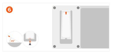
Insert the SSD *(not included)* faceup at a 45-degree angle. Once installed, push down on the SSD and use the silicone pin to keep it in place. Supports NVMe & SATA (up to 10Gbps max speed, 2TB max capacity)
