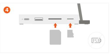
Insert micro or SD cards into card reader slots. Supports UHS-I speeds.
