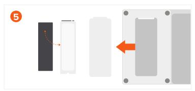
To install the SSD, lift the backside cover on the adapter. Apply the Thermal Pad included to the bottom of the SSD. Ensure pad is properly aligned.
