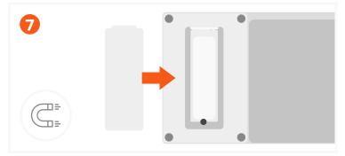
Once the SSD is secured, magnetize the cover back onto the hub.
