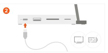
Connect a USB-C drive or peripheral to the USB-C data port (up to 10 Gbps).
