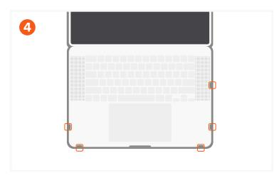
When installing the bottom case, ensure all **5 clips** snap into place.
