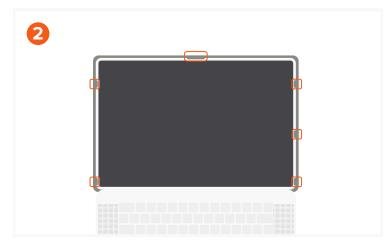
When installing the top case, ensure all **6 clips** snap into place.
