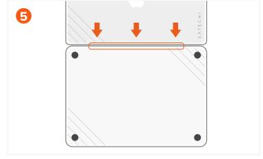
Ensure this long clip snaps into place as well. If it does not snap into place, the case will fall off.
