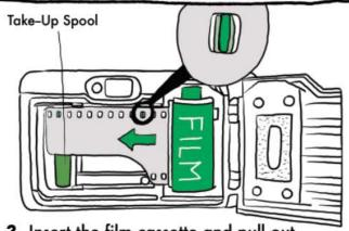
3. Insert the film cassette and pull out a length of film to the left onto the Take-Up Spool. Ensure that the sprocket holes line up with the plastic teeth of the camera.
