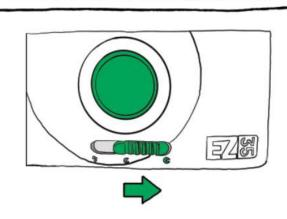
**7.** To preserve battery, move the lens cover switch to the "closed" position after you have finished taking photos.
