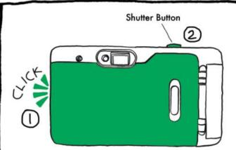
4. (1) Close the camera back firmly with a CLICK. (2) With the lens in the open position press the Shutter Button for the film to auto-wind. Press until the Frame Counter reads '1'.
