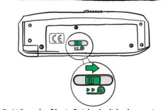
8. When the film is finished, slide the rewind switch (bottom of camera) to the rewind position and the film will automatically rewind. Open the back and remove film for developing.
