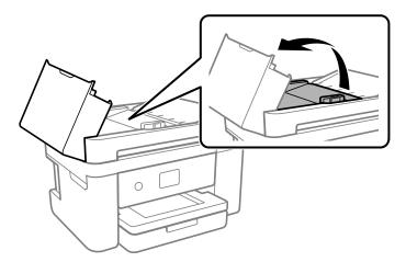
**Caution:** Make sure the ADF cover is opened before raising the ADF input tray or the ADF may be damaged.
