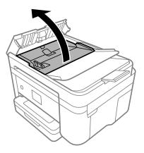
**Caution:** Make sure the ADF cover is opened before raising the ADF input tray or the ADF may be damaged.
