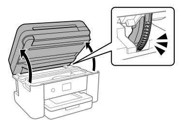
**Caution:** Do not touch the flat white cable or translucent film inside the product. Be careful not to trap your hand or fingers when opening or closing the scanner unit.
