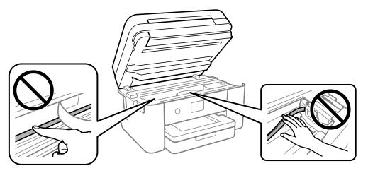
7. Using a cotton swab, wipe off any ink smears on the part shown in the illustration below.
