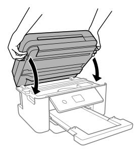
**Note:** The scanner unit is designed to close slowly to avoid catching fingers in the printer. There may be some resistance when closing the scanner unit.
