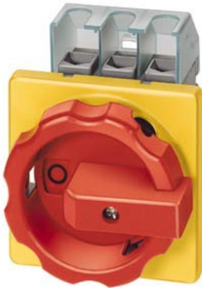
MAIN CONTROL SWITCH 3-POLE IU=32, P/AC-23A AT 400V=11,5KW FRONT MOUNTING FOUR- HOLE MOUNTING ROTARY ACTUATOR BLACK
