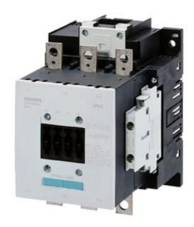
CONTACTOR, 90KW/400V/AC-3, AC(40...60HZ)/DC OPERATION UC 220...240V AUXIL. CONTACTS 2NO+2NC 3-POLE, SIZE S6 BAR CONNECTIONS CONVENT. OPERATING MECHANISM SCREW TERMINAL
