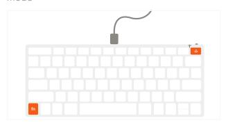
Press and hold one of the keyboard's Bluetooth keys for ~3 seconds, until the LED light starts to blink.
