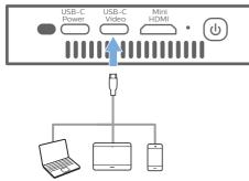
2 The projector automatically switches to USB-C input when a USB-C connection is made. The projection screen shows images.
