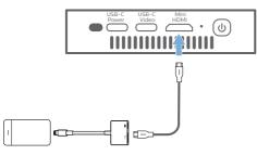
2 The projector automatically switches to HDMI input when HDMI connection is made. The projection screen shows images.
