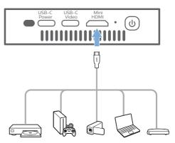
You can also connect an iPhone to the projector. Using the HDMI cable, connect the **Mini HDMI** connector on the projector to the HDMI port on the Apple Digital AV Adapter (not included). Then connect the lightning connector of the adapter to your iPhone.
