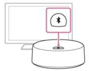
The transmitter is initialized and the pairing information of all the BLUETOOTH devices is deleted. Initializing the transmitter does not delete the pairing information of the neckband speaker.
