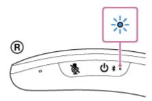
The settings, such as the volume settings, are restored to the factory default settings and the pairing information of all BLUETOOTH devices is deleted. The pairing information of the supplied transmitter is not deleted in the course of initialization.
