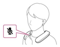
While a phone conversation is in progress, pressing the (microphone off) button triggers voice guidance (Mic OFF) indicating that the microphone is turned off. When you press the button once again, you hear voice guidance (Mic ON) indicating that the microphone is turned on.
