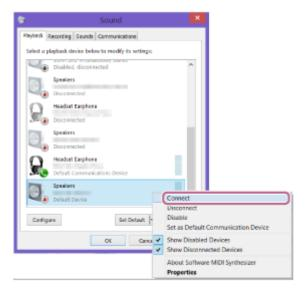
When the neckband speaker is connected, a checkmark will appear on [SRS-NS7 Stereo] on the [Sound] screen. Proceed to step 3 .
