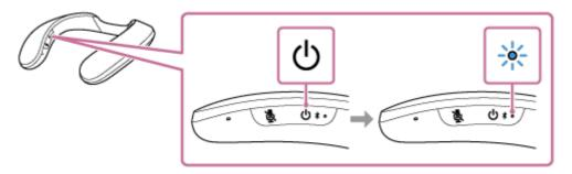
When a BLUETOOTH connection is established with the previously connected device, you hear voice guidance (BLUETOOTH connected).
