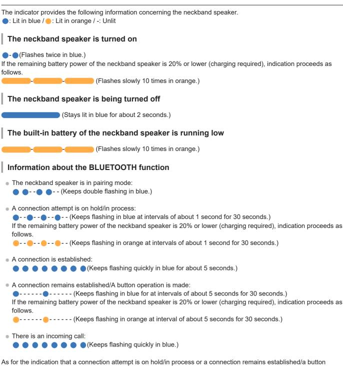
As for the indication that a connection attempt is on hold/in process or a connection remains established/a button operation is made, the indicator automatically goes out in a predefined period of time. When any operation is performed on the neckband speaker, the indicator, once again, keeps flashing for a predefined period of time.
