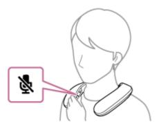
While a phone conversation is in progress, pressing the (microphone off) button triggers voice guidance (Mic OFF) indicating that the microphone is turned off. When you press the button once again, you hear voice guidance (Mic ON) indicating that the microphone is turned on.
