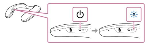
When a BLUETOOTH connection is established with the previously connected device, you hear voice guidance (BLUETOOTH connected).
