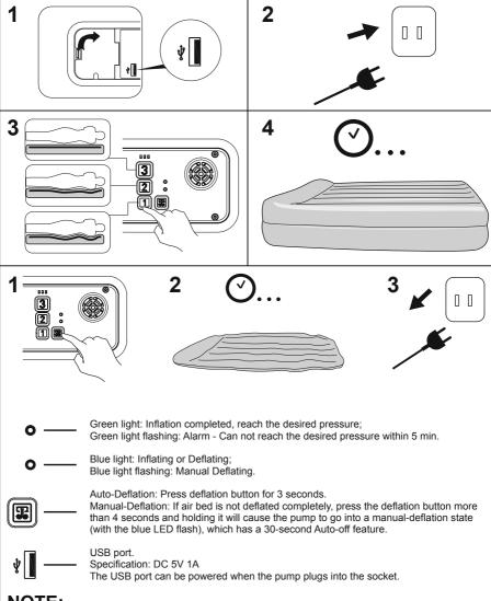
**NOTE:** When all 3 power buttons are flashing this indicates one of two things: 1) The power is on, or 2) The power has been off and is now reconnected to a power source. This pump has an auto-re-inflation feature. Please keep the pump plugged in and make sure the green light is on to maintain the air pressure level that you choose.
